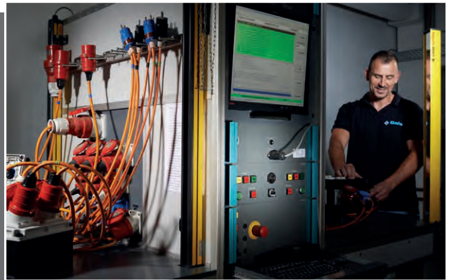
Fully automatic testing station with documentation
