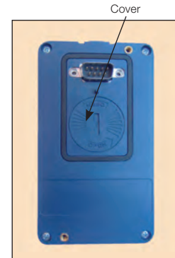
Figure 31: Keypad battery cover to access battery
