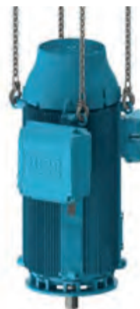
Figure 4.9 - Lifting of HGF and W50 motors.
