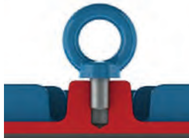
Figure 4.2 - Incorrect tightening of the eyebolt
