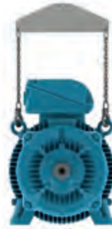
Figure 4.7 - Use of a spreader beam for lifting
