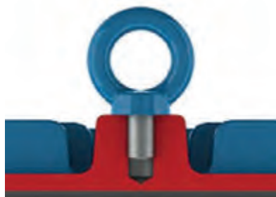
Figure 4.1 - Correct tightening of the eyebolt
